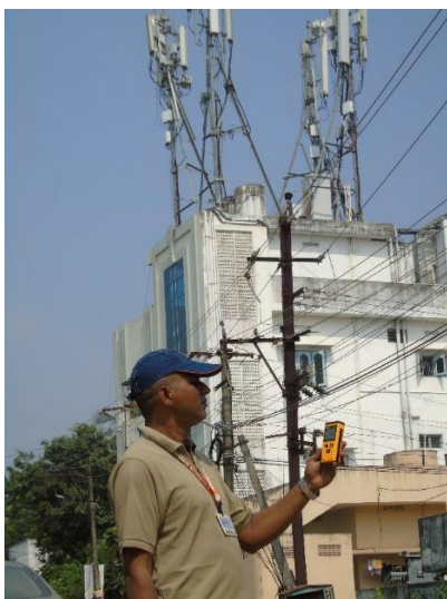
Fig.3. Measuring strength of EMR at Rajula colony cellular antennae
